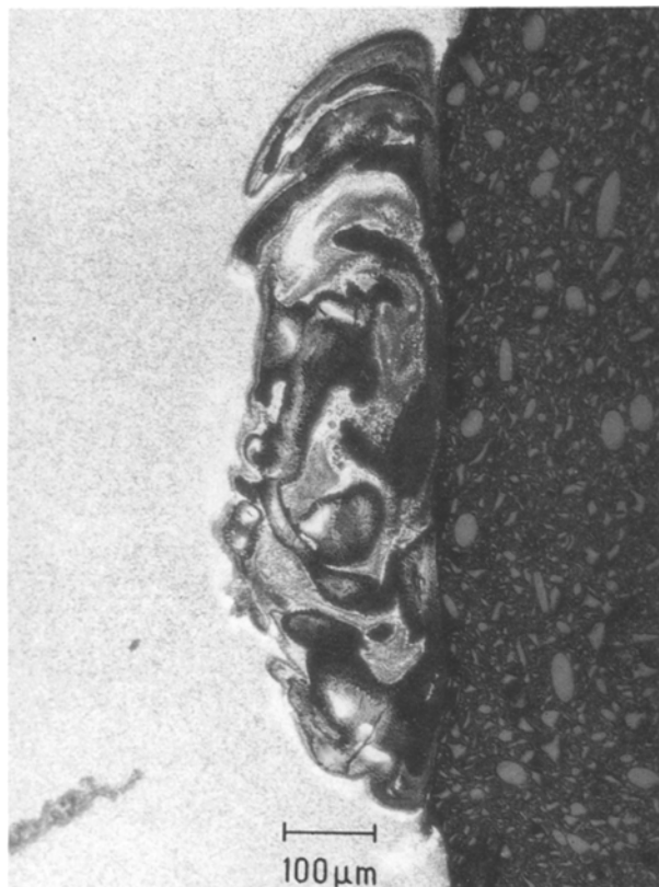
Figure 3 Manganese on aluminium; “onion scale” type layers. Scanning velocity 10 \text{ cm sec}^{-1} .
