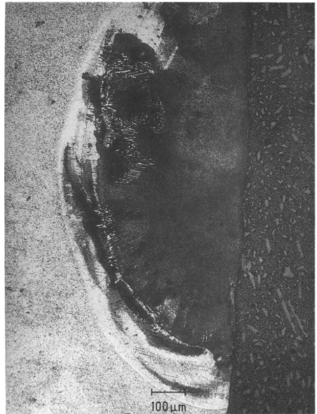
Figure 4 Manganese on aluminium; cross-section after two laser passes at the same place. Scanning velocity 1 \text{ cm sec}^{-1} .
